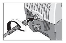
**Step 1**Connect the high pressure hose to the unit's high pressure outlet.
